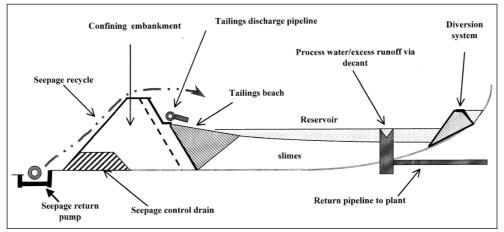
Figure 1. Schematic cross-section through a TMF
