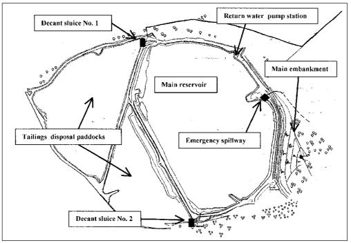
Figure 4. Blakedon Hollow Tailings Dam (Drawing courtesy of Glebe Mines Ltd)
