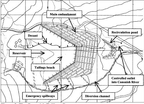
Figure 3. The Cononish Tailings Dam (Drawing courtesy of AMEC Earth and Environmental Ltd)
